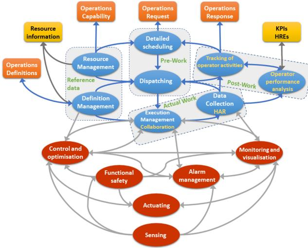
Fig. 2. Activity model of manufacturing operations management with an operator-centric view
