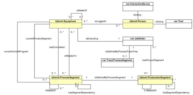
Fig. 5. Implementation of B2MML elements in the Dynamic Actual Status Representation of VAR Ontology [37]
