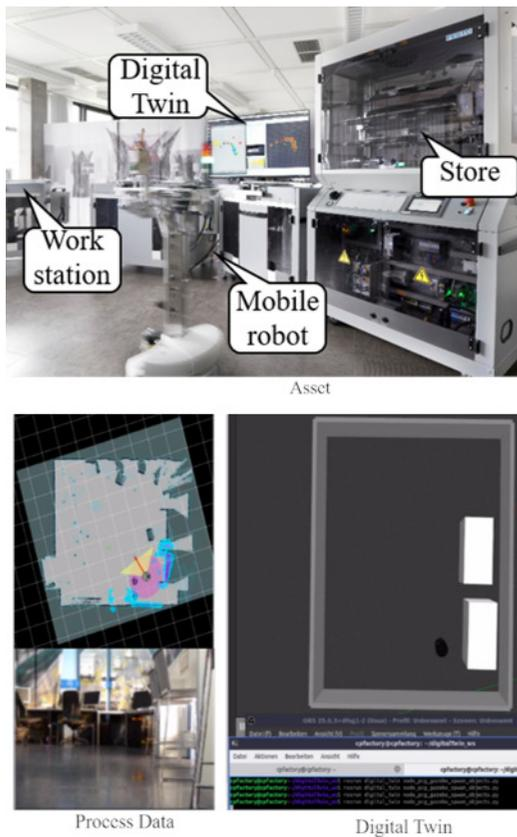
**Fig. 6** Visualization of the Cobot and its intelligent Digital Twin
