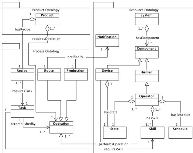
Fig. 6. Structure of an ontology, for Including Human Tasks as Semantic Resources in Manufacturing [44]
